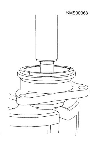
CHECKING AND REPAIRING COMPONENTS Checking commutator end shield Check bushing for damage and running marks. Removal: Use pressing-out and pressing-in mandrel to press out bushing. Pressing-out and pressing-in mandrel for bushing in commutator end shield: 0 986 617 190
